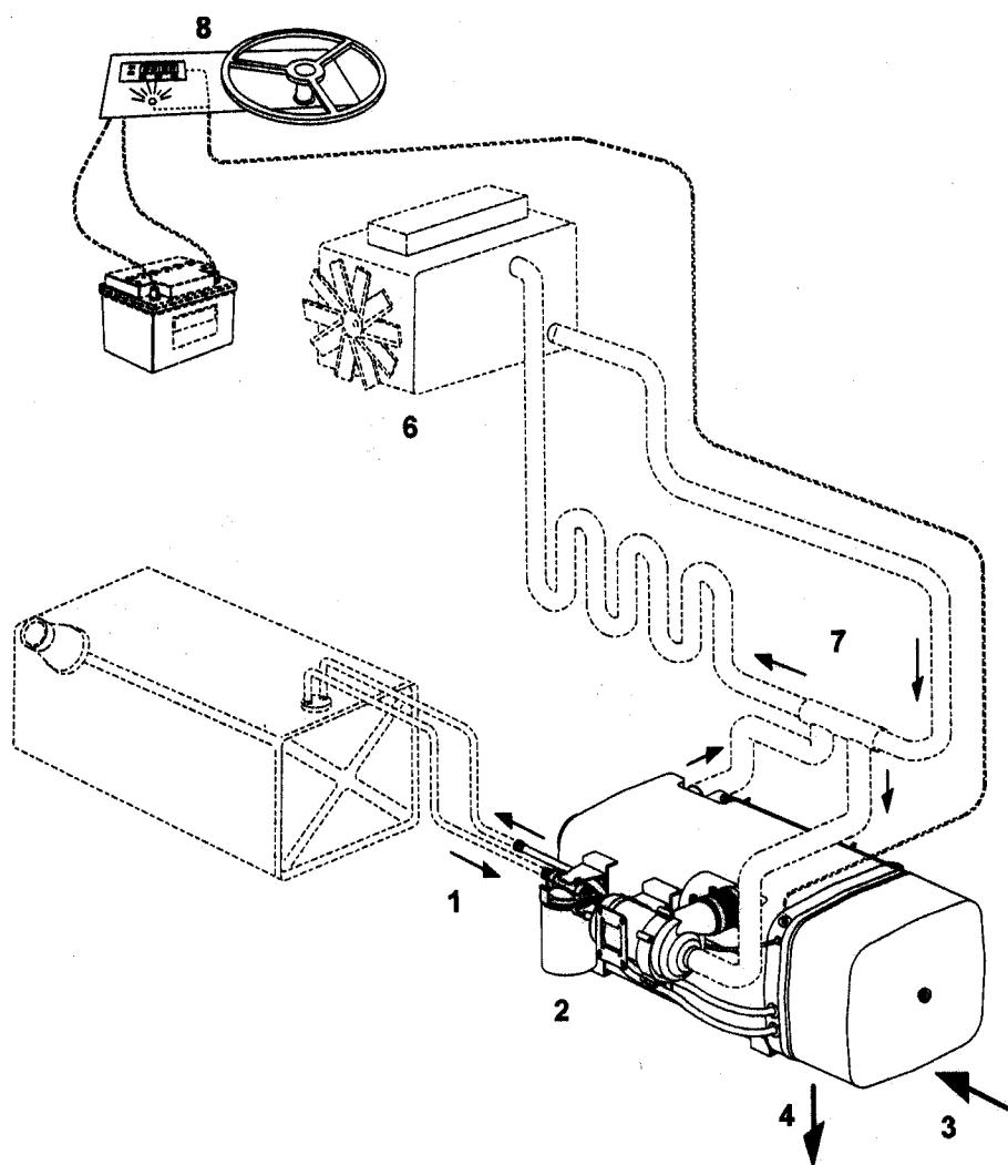
1:Dieselolje, 2:Filter, 3:Luft, 4:Utblåsing, 6:Motor, 7:Varmesystem, 8:Kontrollpanel
